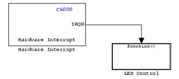
In this model, the Hardware Interrupt block installs a task that runs when it detects an external interrupt. This task then toggles an external LED on or off.
